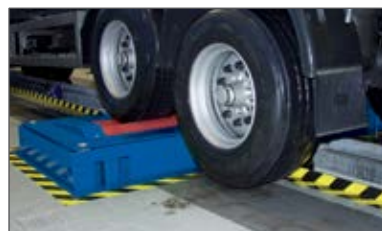
Roller set lifting Hydraulic roller set lifting for axle load displacement on the axle being tested.
